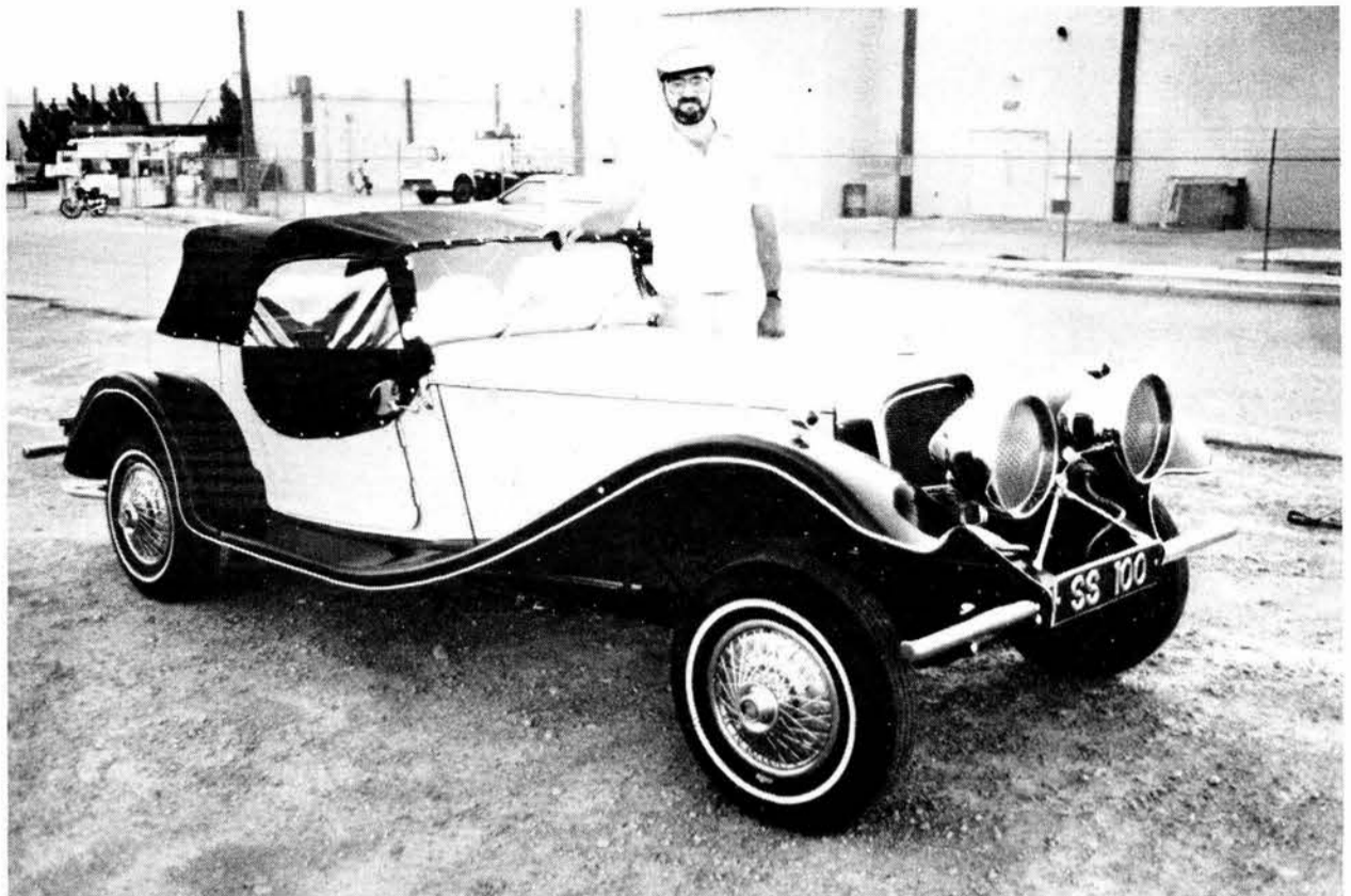
LAS VEGAS EYE-CATCHER — Diwiatt Barker (7171) displays his classic replica of a 1937 Jaguar SS100 that he built from a kit. The SS on the license stands for the Swallow Sidecar Company of England (forerunner to the Jaguar name); the 100 designates 100 mph. Only 309 of the machines were built in 1935-40. Diwiatt's car has a '74 Pinto engine and transmission.
